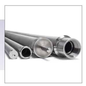
Our septa filter elements are made from Sinterflo® mesh composite (MC) filter media. This unique material is made from wire mesh and perforated metal, sintered together into a durable porous filtration medium.
